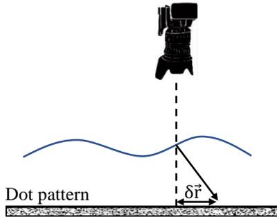
Figure C1. A distortion of the random dot pattern. As waves appear at the surface of the liquid, light-rays reaching each one of the camera pixels will have a slightly different origin compared to the reference image (according to Snell's law), and the image will appear to be distorted.
