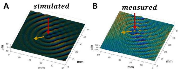
**Figure 6.** A comparison between the measured wavefield created by a walker (right) and a simulation of the wavefield (left). Red arrows indicate the location of the previous bounce of the droplet, and yellow arrows indicate its direction of propagation. Measurements were made at forcing amplitude of  $\gamma = 4.11 \pm 0.02$
