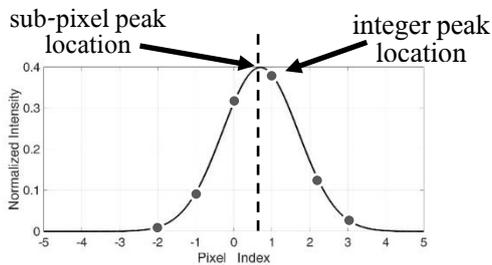
Figure C2. Sub-pixel estimation of the displacement field. The dot-pattern beneath the liquid was put through a gaussian filter – each dot had maximum darkness in its middle and decayed to white in a gaussian form. The PIVLab algorithm could now estimate the gaussian's maximum and retrieve sub-pixel resolution.
