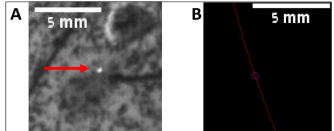
Figure A1. Measuring the path of walkers. (A) A spotlight was held at 45° to the bath, allowing mostly the reflection of the droplet to reach the camera, which made the droplets shine compared to their background. (B) The location of the droplet was recorded in every frame using TrackMate add-in for ImageJ. Images were taken at 160fps (4 times the bouncing frequency)
