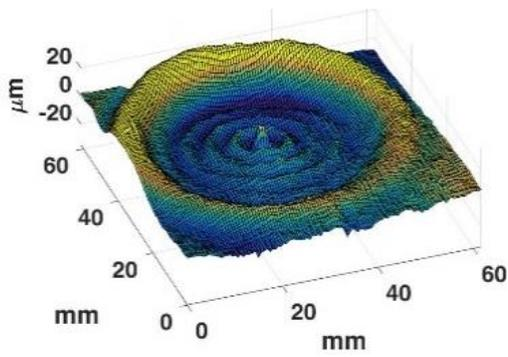
Figure B1. A Traveling wave of circular form was created after disturbing the liquid surface using a toothpick. Images were taken at 1,000 fps.
