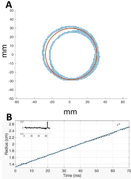
Figure B2. Measuring the radius of the circular traveling wave. (A) A circle was fitted to the mid-height of the traveling wave. (B) Measuring the radius of the traveling wave increase of time can allow us to measure the speed of propagation. A linear increase in radius was measured.
