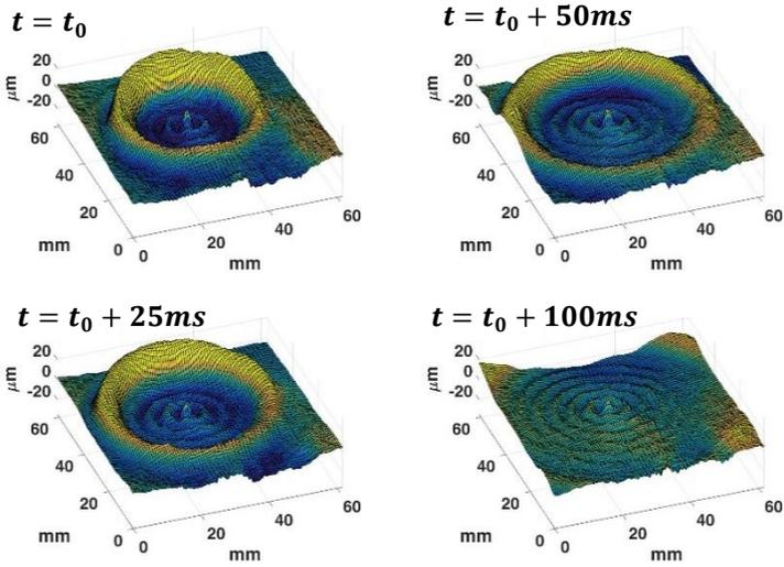
Figure 3. The time evolution of the wavefield after a single impact caused by a toothpick. The top-left image was captured at  $t_0 \approx 150ms$  following the impact. The system was driven at 80Hz and amplitude  $\gamma = 4.12 \pm 0.02$ . Images were taken at 1,000 fps.
