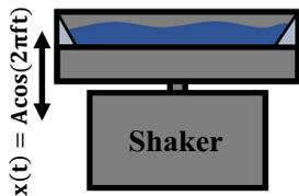
Figure 1. The experimental setup. A circular vessel was attached to a shaker, which was set to vibrate in sinusoidal waveform. The vessel's walls were coated with silicone seal to minimize boundary effects.
