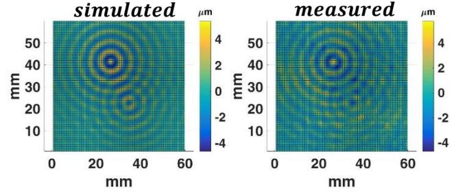
**Figure 5.** A comparison between the measured wavefield of a double-toothpick impact (right), and the superposition of two distinct standing waves as modeled in the previous sections (left). The measured wavefield is the field present at the surface after the traveling wave has left the ROI. Measurements were made at 80Hz, while the acceleration amplitude was  $\gamma = 4.14 \pm 0.02$ .
