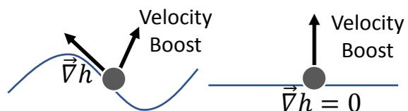
Figure 2. A diagram showing how momentum could pass to the droplet not only vertically (due to the parametric oscillations), but also horizontally when the gradient field is non-zero ( $\vec{\nabla}h \neq 0$ ).
